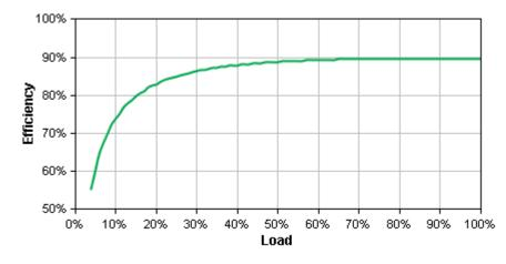
Curve fit to measured efficiency data. All measurements taken in normal operating mode, at typical environmental conditions, with nominal electrical input and resistive load output.
